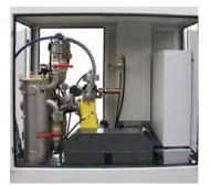
Stationary electric unit with sound damping cover
