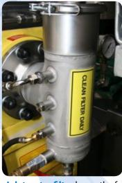
• Inlet water filter keeps the feed supply water clean, extending the life of key components within the pump, nozzle and jetting guns. The simple design allows quick replacement of filter.
