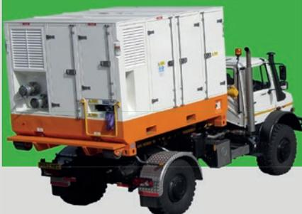
**Built for the nuclear industry**, this is one of 12 lightweight pump units designed for transport by off-road vehicle. The units are reactor cooling water flood pumps for emergency response at various installations across the UK.
