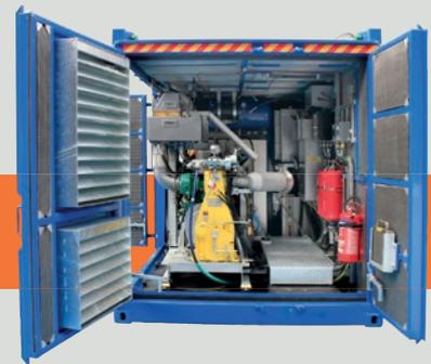
**The container-mounted diesel unit** has the same options as the electric version. Specific features of this unit include external fuel fill, and gas & fire suppression. These units can be Rigsafe, Atex Zone 2, or NORSOK compliant.
