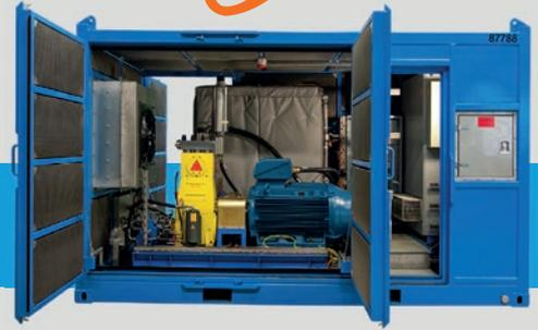
**CSC, Std ISO, or DNV-approved** containers offer maximum protection and security. Options include noise attenuation, integral control room, internal lighting, and storage. Ideal for onsite security and global mobilisation. These electric units can be supplied as ATEX Zone 1 hazardous area compliant.
