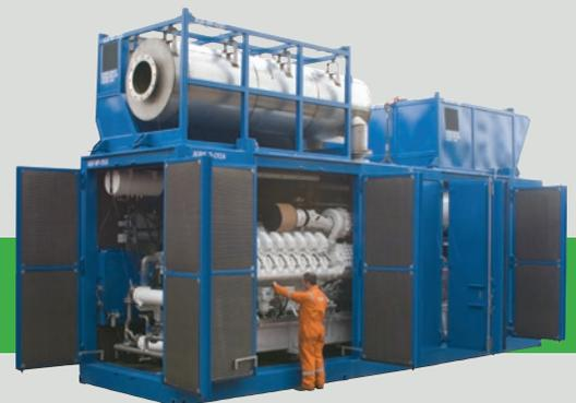
**Designed for a very high flow application**, this monster pump unit was one of three designed, built, and manufactured by Calder for subsea trenching from a barge.
