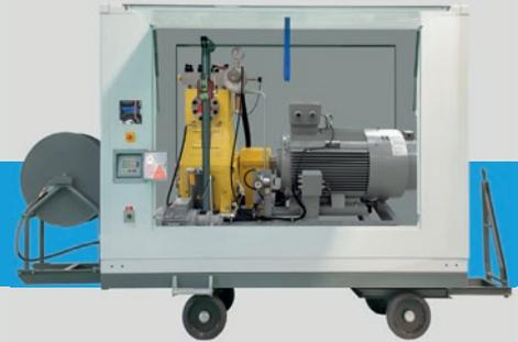
**This trailer-mounted, road-going electric pump unit** can be towed into position. Ideal for multi-site use or semi-permanent installation.
