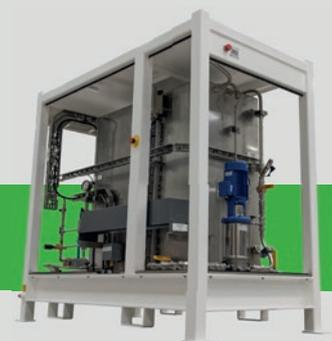
**This unit delivers a specific,** measured flow of water for nuclear decontamination. It has low pressure, pre-wash and high pressure, full clean settings.
