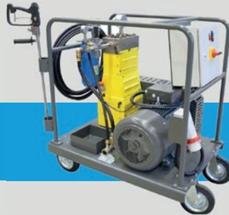
**Lightweight, trolley mounted units** can be wheeled into position and plugged into local power points. It produces pressures up to 3,000 bar.
