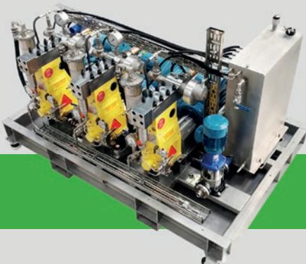
**This triple pump unit** was designed for a customer with severe space constraints. The design maximises the use of space whilst maintaining serviceability.
