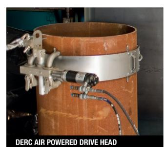
The DERC Air Powered Drive Head moves the cutting nozzle across the surface, creating a cut at a constant rate of speed.
