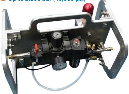
Air return signal from the gun return line is connected to the pneumatic cylinder. When triggers are pulled, air is applied to the cylinder closing the 'dump' valve and pressurising the gun. When triggers are opened/ released air is vented from the cylinder and the gun is depressurised. Our fail-safe design allows depressurisation if air hoses leak or burst. High pressure wear parts can be field-replaced in minutes courtesy of the cartridge repair kit.
