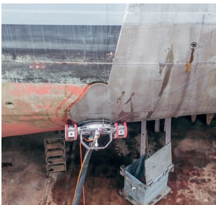
The Spiderjet® V is held on the work surface by a vacuum, which at the same time suctions off the removed waste material and waste water.
