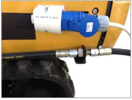
Easy connection to high pressure pump unit via bulkhead connector.
