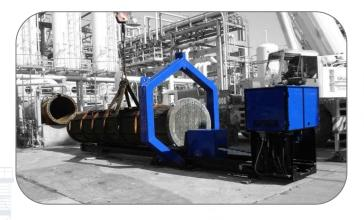
This versatile, remotely controlled extractor is designed for manoeuvrability. This self-
