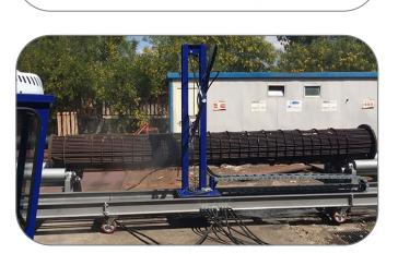
The IdroBox is a lightweight, internal tube cleaner. It is a modular system which can be configured to clean three tubes at a time. Simple remote-control operation with positioning XY option.
