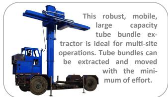
This hook-lift extractor's tube pull/push operations are achieved through its integrated power unit. Hydraulic operation is through remote control. A self-balance capability ensures the load and machine are balanced.
