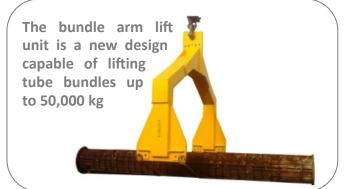
Our bundle handling equipment includes versatile extractors and movers for the removal and re-insertion of bundles both large and small. Our bundle movers range from the simple lift arm to the mobile straddle carrier.
