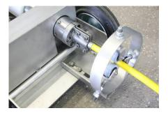
The rotating unit is driven by 120 Nm³ / hr. of compressed air at 4 bar and comprises a pneumatic motor with gearbox, a pneumatic maintenance unit, the high pressure rotary joint and a pneumatic control system all mounted on a 3 wheel trolley.
