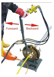
The hose deployment unit is mounted on a sturdy base plate and comprises the height adjustable control lever to deploy or retract the hose which incorporated the remote control to operate the hose rotating unit.
