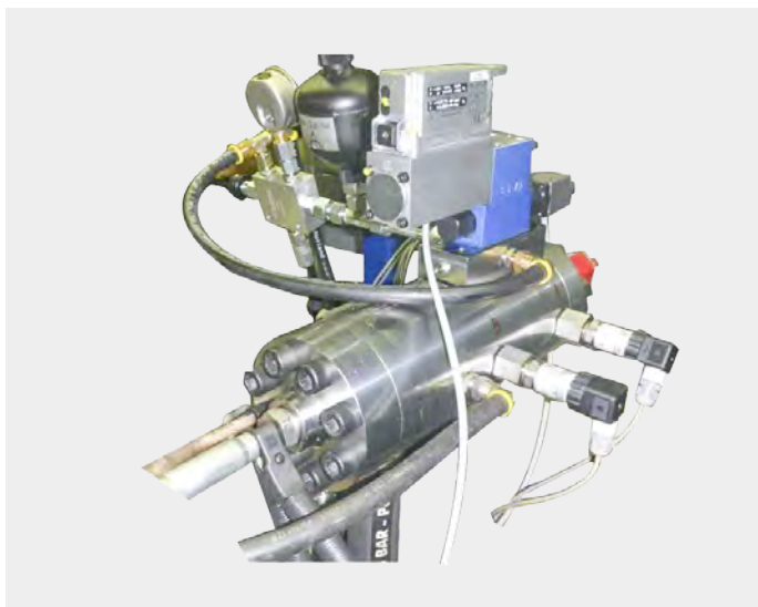
Pressure regulating valve with servo control
