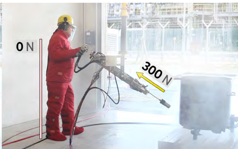
Reaction force free working with JETMATE
