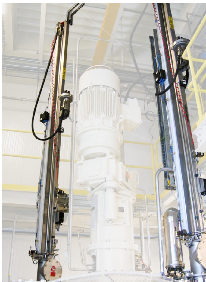
Lance system - moved pneumatically actuated
