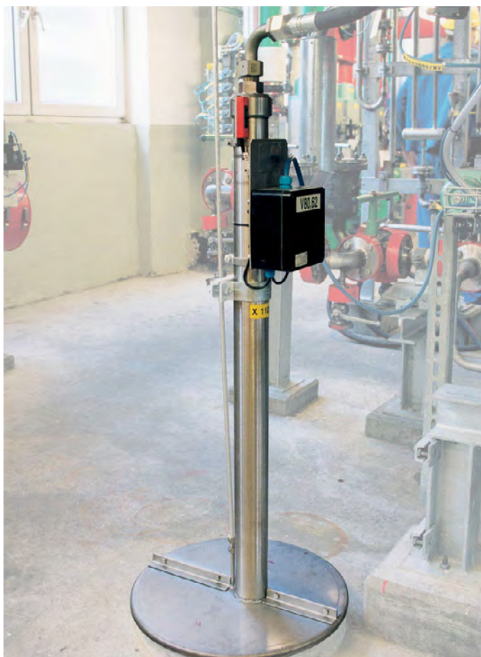
Lance system - moved hydraulically/pneumatically actuated
