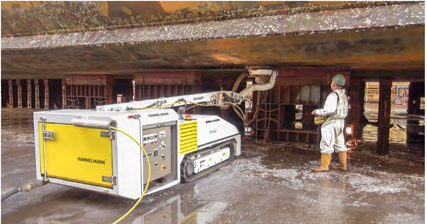
The Dockboy is a modern tracked vehicle primarily for working on ship hull bottoms or similar surfaces.
