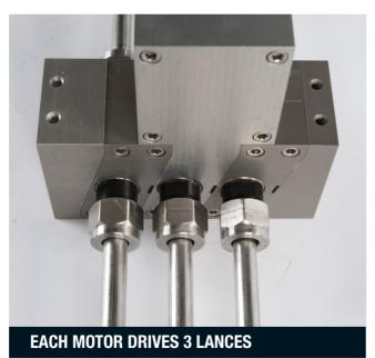
The basic drive module includes a motor (air or hydraulic driven), powering the rotation of the lance with a maximum of 600 rpm. Each motor of this basic drive module can rotate up to three lances. By adding modular extension blocks, you are able to choose how many lances you wish to apply.
